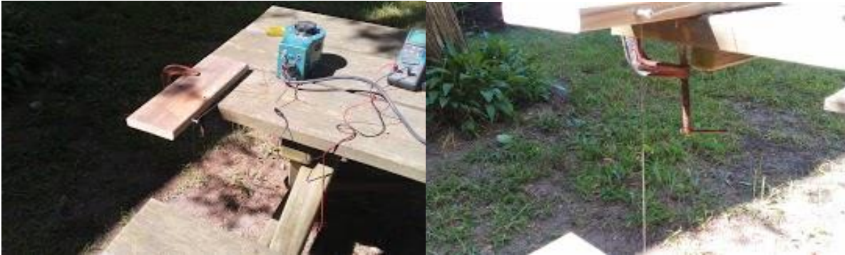
Hotwire cutter with Variac and Current Meter
