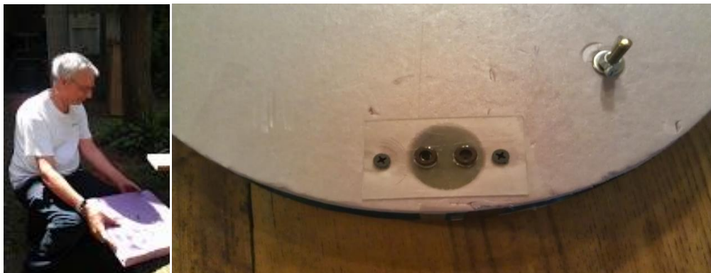
Cutting the Round Coil Form from a Square Piece of Rigid Foam Insulation
