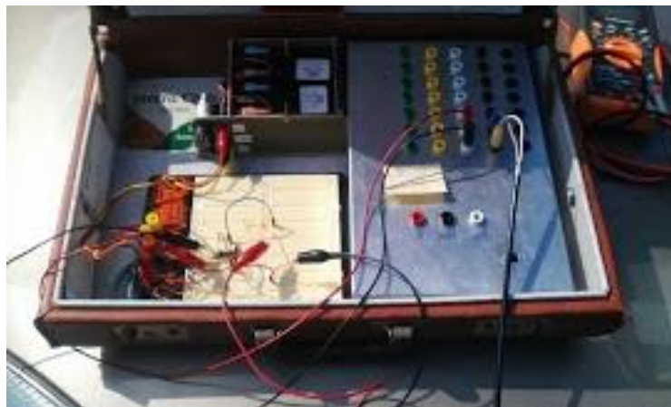
Briefcase Field Setup: Prototype pre-amp shown
