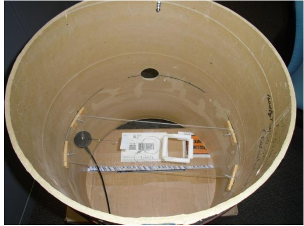
Sense Coil Mounted to Fixture Inside Helmholtz Coil (20 cm position)
