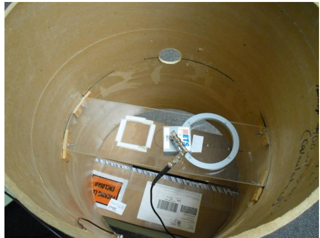
ETS Lindgren 7604 Loop Antenna Inside Helmholtz Coil
