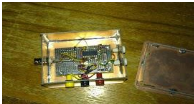
INA103 Pre-Amplifier in Shielded Enclosure
